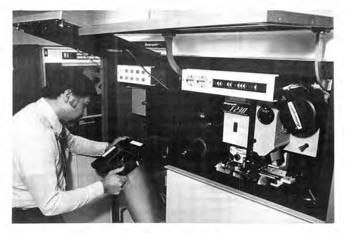
OPERATOR Joe Tapia (5411) inspects the cathode ray tube of the new 4460 computer during installation in Sandia's Computing Center in Bldg. 880. The new system provides increased capabilities in computer created graphics, including animated motion pictures and automatic production of microfiche and aperture cards.
